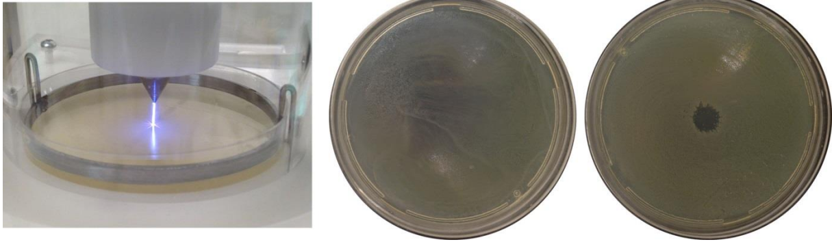
Figure 2. Irreversible electroporation of E. coli with ten discharges of approx. 100 A peak current. (a) The exposure. (b) The control plate (loaded into the system, but no discharge applied). (c) The exposed plate. The transparent areas correspond to regions with absence of E. coli colonies.
